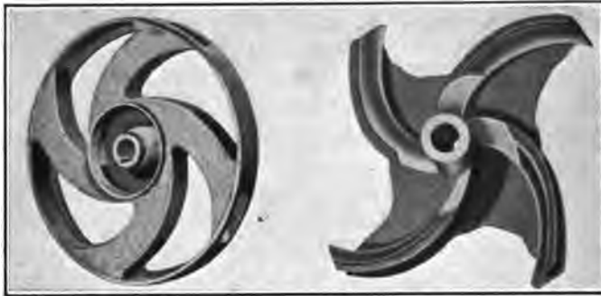
Hollow arm impeller.
